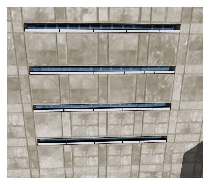
The strip lights will be mounted at the top and bottom of the front edges of each of the 4 window sills. These lights will be focused at a 45 degree angle inwards towards the window. This will cut down on glare while still illuminating the window sills.
