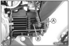
A. Spark Plug Cap B. Spark Plug
