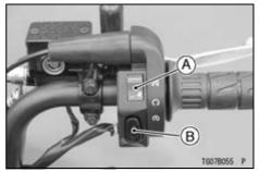
A. Engine Stop Switch B. Starter Button
