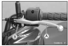
A. Clutch Lever B. Starter Lockout Switch
