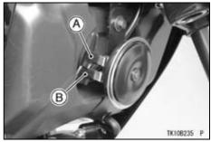
A. Horn Lead Connector (Brown/White Lead) B. Horn Lead Connector (Black Lead)
