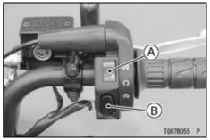
A. Engine Stop Switch B. Starter Button
