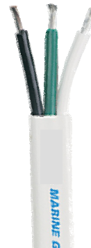
Boat Cable, White outer jacket (105° C dry, 75° C wet, Rated to 600 volts, Meets DOT & USCG Specs)
