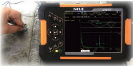
Dynamic beam tracking to visualize the flaw location
