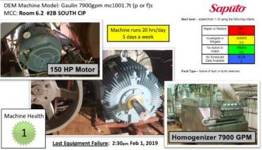
Installed new motor and re-started machine on Friday Feb 1, 2019 @ 6:30pm
