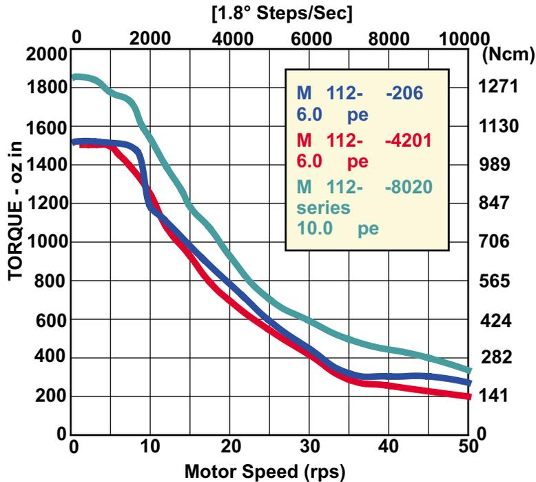
◆ Duty cycle is dependent on torque, speed, Drive parameters, and heat sink conditions. Maximum case temperature is 100°C.
