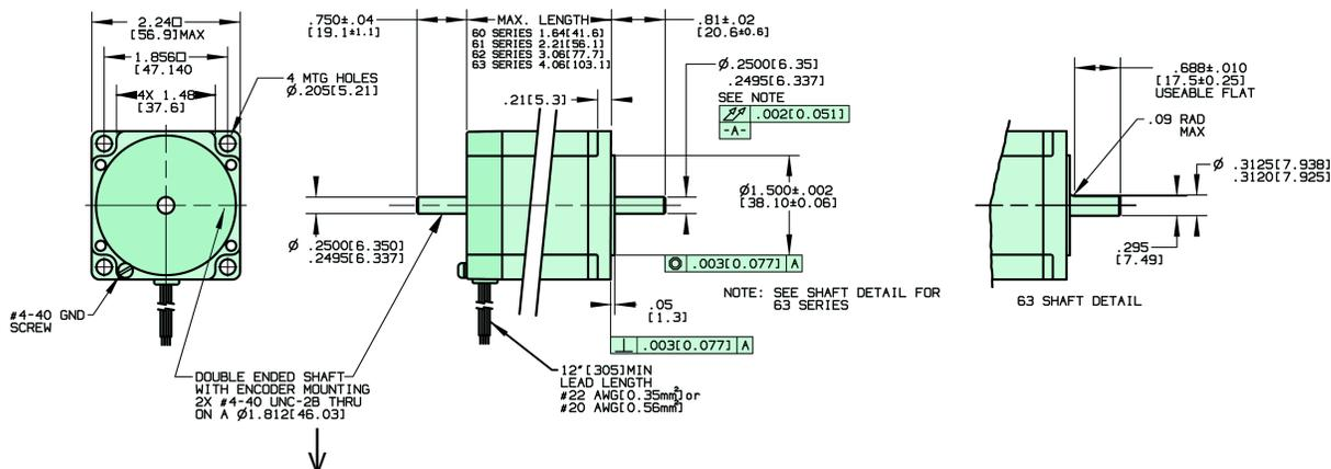
Add "E" to model number for double ended shaft. Example: KML062F07E
