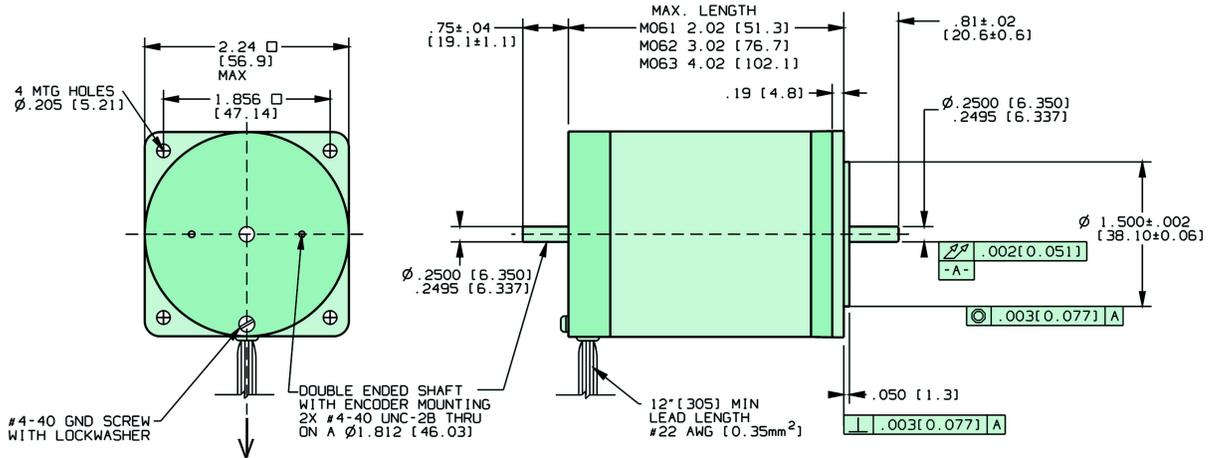
Add "E" to model number for double ended shaft. Example: M062-LS03E
