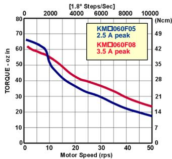
◆ The curves do not show system resonances which will vary with system mechanical parameters.
