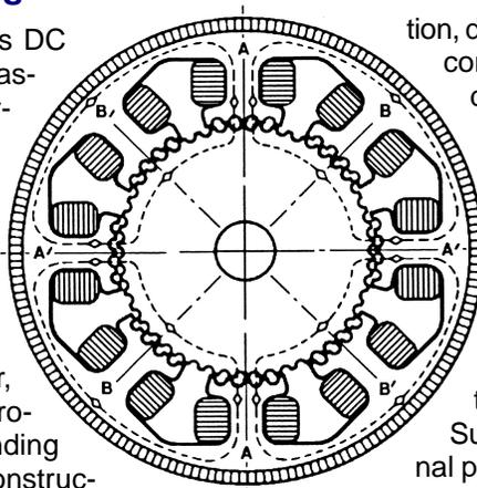
tion, deliver a 1.8° step angle. Both configurations have a slightly different tooth pitch on the stator (48 or 52) to provide smoother operation and softer step-to-step motion with less resonance or mechanical instability at low speed. The 52 tooth stator design is used in the new KM06 and KM09 motors to provide extra torque. Superior Electric held the original patent on the 48-50 design.
