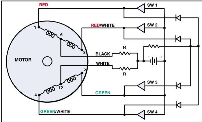
**Note:** Circuit shown is only for use with a unipolar drive
