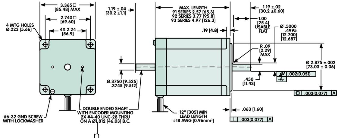
Add "E" to model number for double ended shaft. Example: KML092F07E
