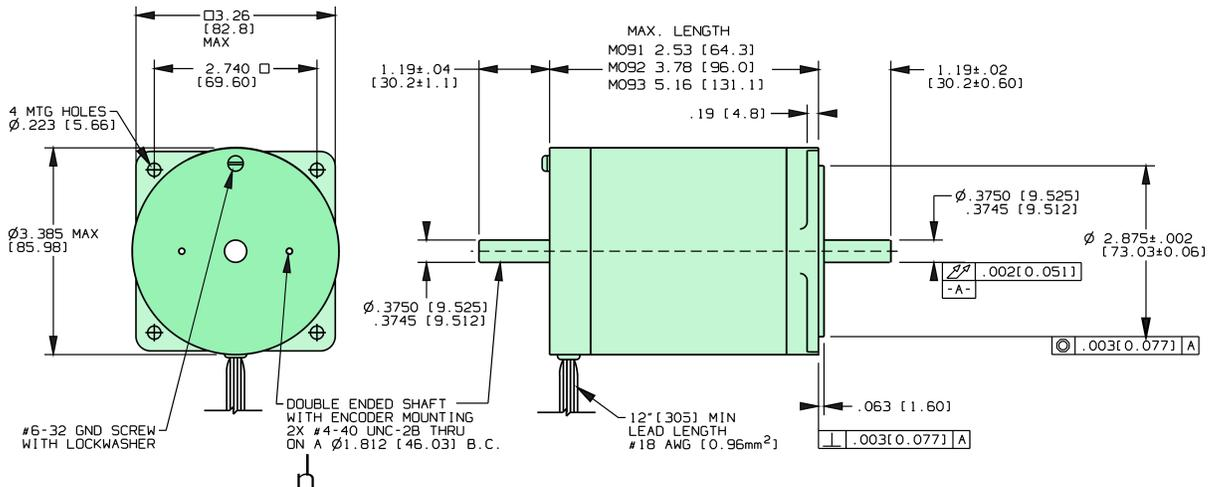
**Add "E" to model number for double ended shaft. Example: M092-LS08E**
