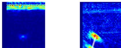
**Figure 2.** Training DPS data set: typical TFM and MTFM images of the buried notch
