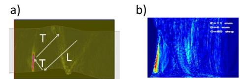
**Figure 3.** The back wall crack imaged (using the half-skip LTT mode) with a) CIVA and b) the AutoNDE code.
