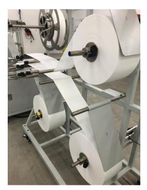
Three layers of electrostatically-charged media.
