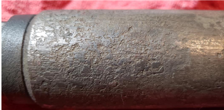
Figure 6: delaminated SM coupling
